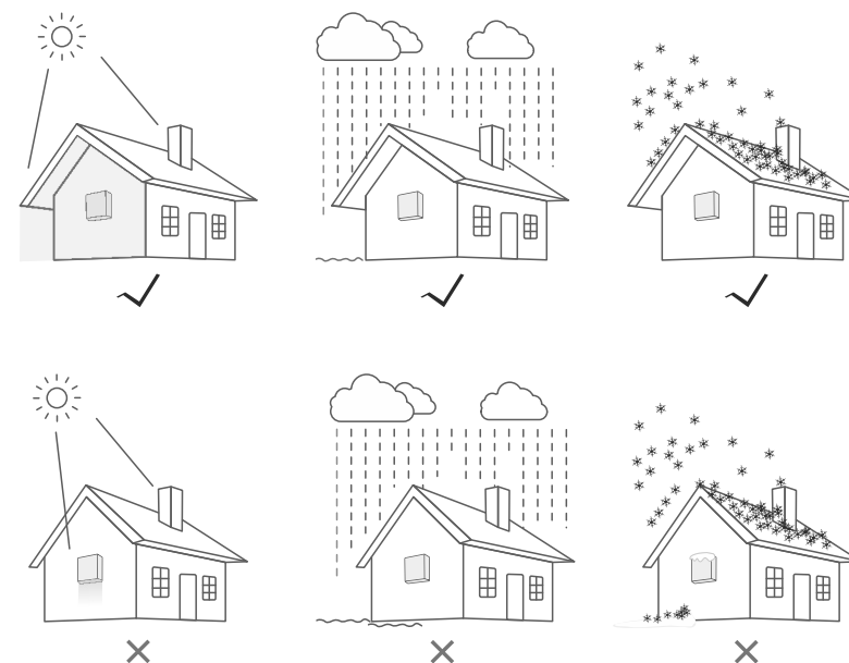
▲ Figure 4.1 Recommended Installation locations
