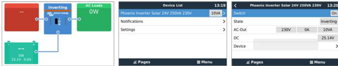
Example of GX screens from left to right: system screen, device list and inverter device screen.
