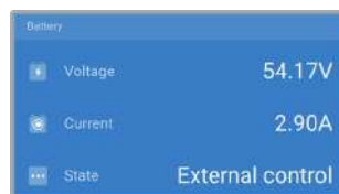
The VictronConnect app indicating that the charger is externally controlled.
