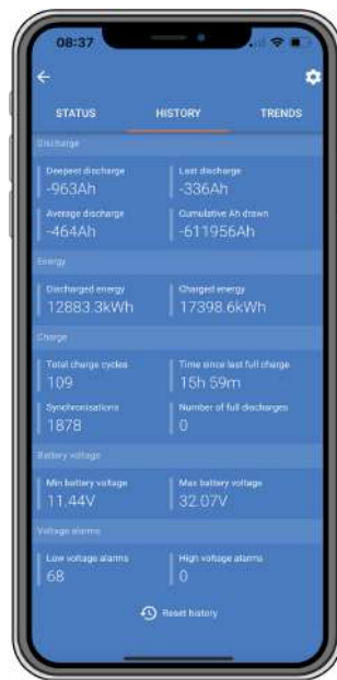
VictronConnect app showing battery monitor history
