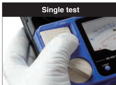
Measurement voltage is applied while MEASURE key is pressed
