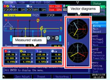
Verify that the connections are correct, referring to the vector diagrams and measured values on the [Wiring] screen.
