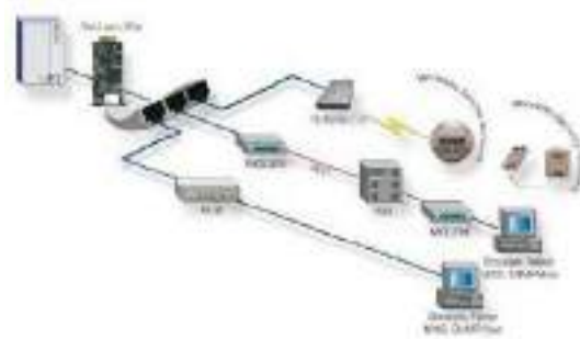
Typical topology of the UPS Network Management
