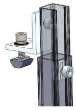
4. Use fixing nuts to attach rail to adjustable rear leg. Tighten M8 hexagon screw securely.
