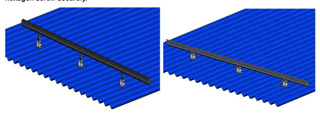
3. Also In accordance with the planned array layout, place the adjustable rear support feet and legs in position using the EPDM waterproof gaskets between the foot and the roof material,
