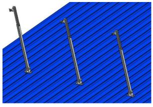
Adjust the size of the rear leg assembly by extending the central angle bar to the desired length. Use the supplied fixing nuts to secure the two sections in place.
