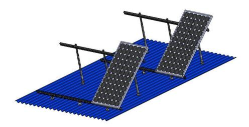
6. Use end clamps with M8\*25 Hexagon screw and fixing nuts to attach solar panels to the rails. Adjacent solar panels are attached by using mid clamps with M8 Hexagon screws.
