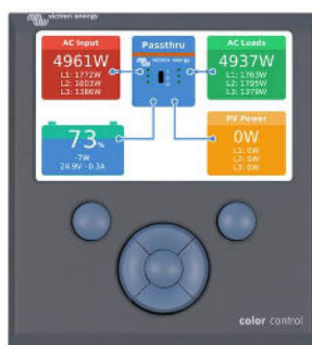
Color Control GX, showing a PV application
